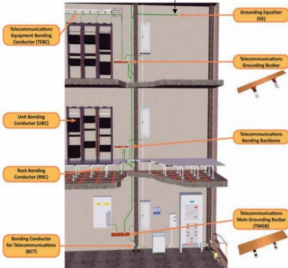
Main components of the telecommunications bonding and grounding system
