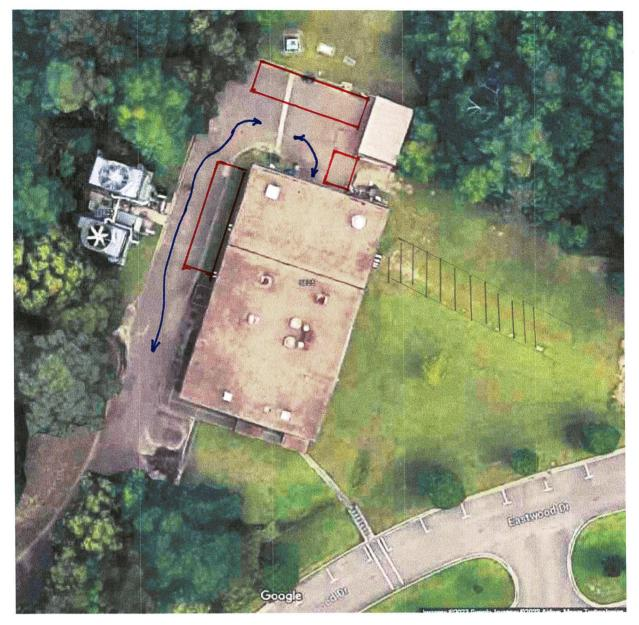
In general, the contractor is responsible for protecting all underground utilities. However, on the <u>Power</u> <u>Plant Building</u>, the protection of underground utilities is particularly important. There are underground hot and cold-water supply piping on the east side of this building under the berm that is visible. This area must be protected at all times from vehicular traffic.
