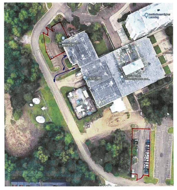
The primary Staging Area for this project will be the parking lot that is south of the **ETV 2 and ETV 3 Buildings**. Fencing will be required to enclose this area with gates at the south end. The north most portion of this lot will be used by a mechanical contractor that is working in the penthouse of the ETV 1 building (a separate project from this roofing project), so this portion of the parking lot will not be available for use by the roofing contractor.
