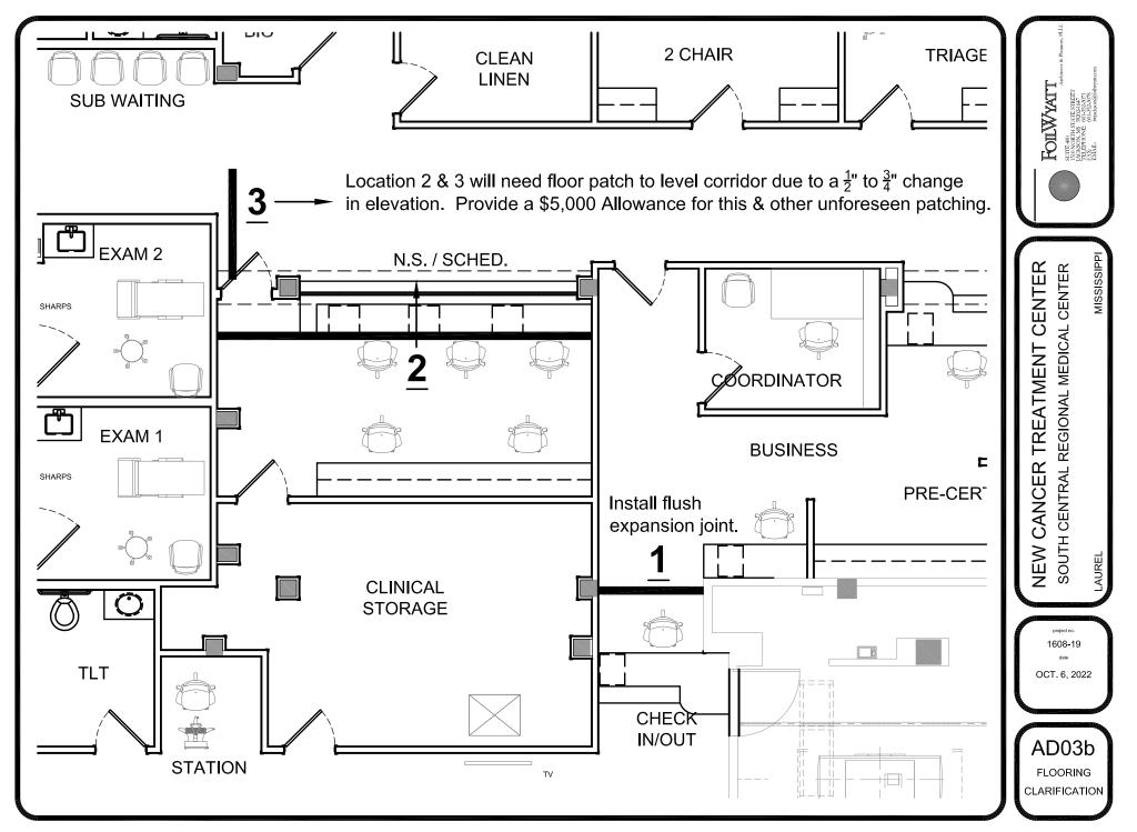
Existing Decon room floor shall be grinded & made level to accept new VCT01 in room 1031.
