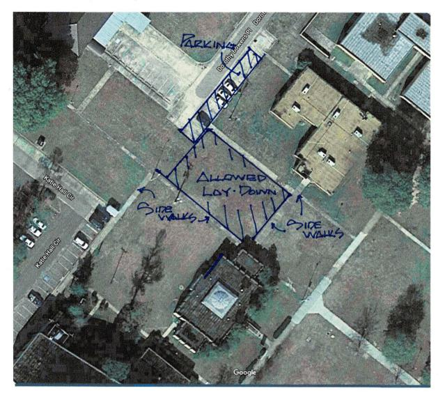
Note the location of the allowable Laydown/Staging area. The contractor will be allowed to use as much or as little of this area that he needs. However, any area used to store materials, equipment, etc. must be enclosed by fencing with windscreen. Gates are to be installed as necessary for the contractors use and access. All disturbed grassed (turf) areas are to be leveled and reseeded once work is complete.
